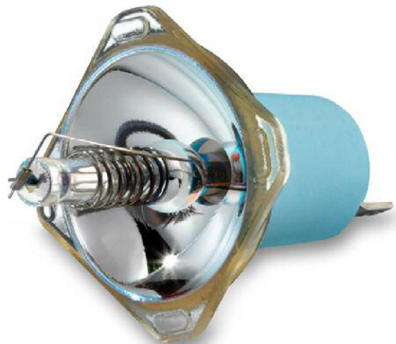
Figure 40. Photo of the BAMI lamp. The back reflection principle allows for a reflector as small as 33 \times 33 \text{ mm}^2 . The antenna spiral for the low voltage ignition can be seen.
